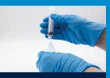
3 Screw a disposable, sterile plastic or glass syringe with male Luer-lock connection fitting (not provided with the device) directly to ampoule.
